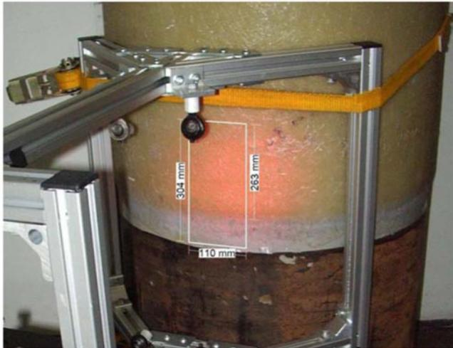
**Figure 3.** The authors created an artificial delamination in this repaired gas pipe.
