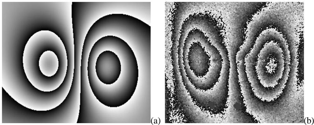
Figure 3: Typical shearographic pattern: (a) Simulated image, (b) Real image
