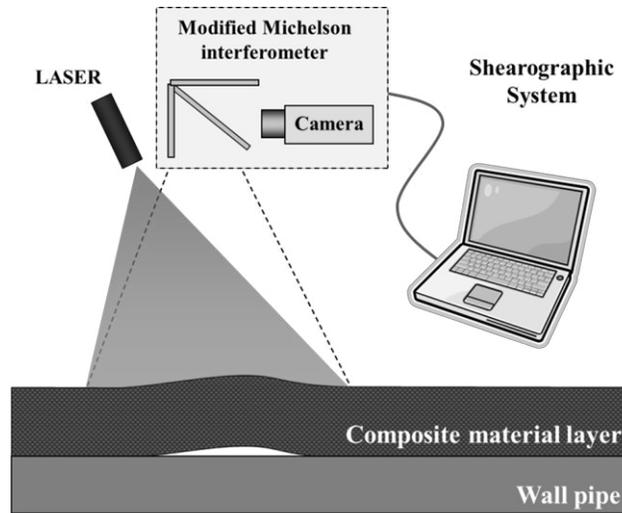
Figure 1: Shearographic setup
