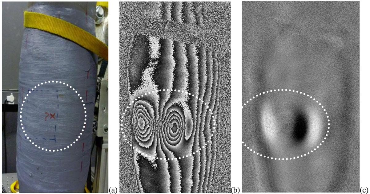
Figure 9: (a) Real composite sleeve; (b) Phase map obtained with shearography and pressure excitation; (c) Map obtained with the proposed method
