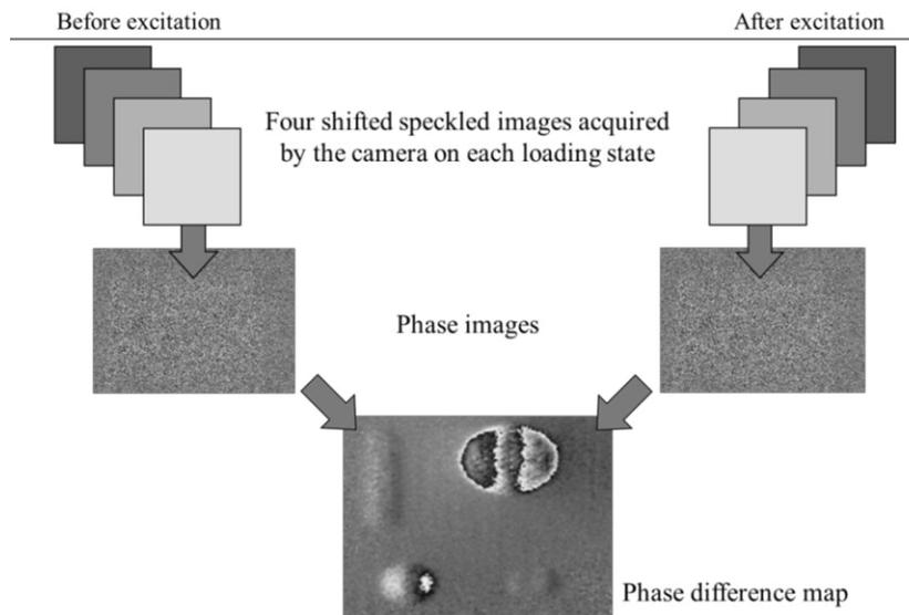
Figure 2: Shearographic inspection
