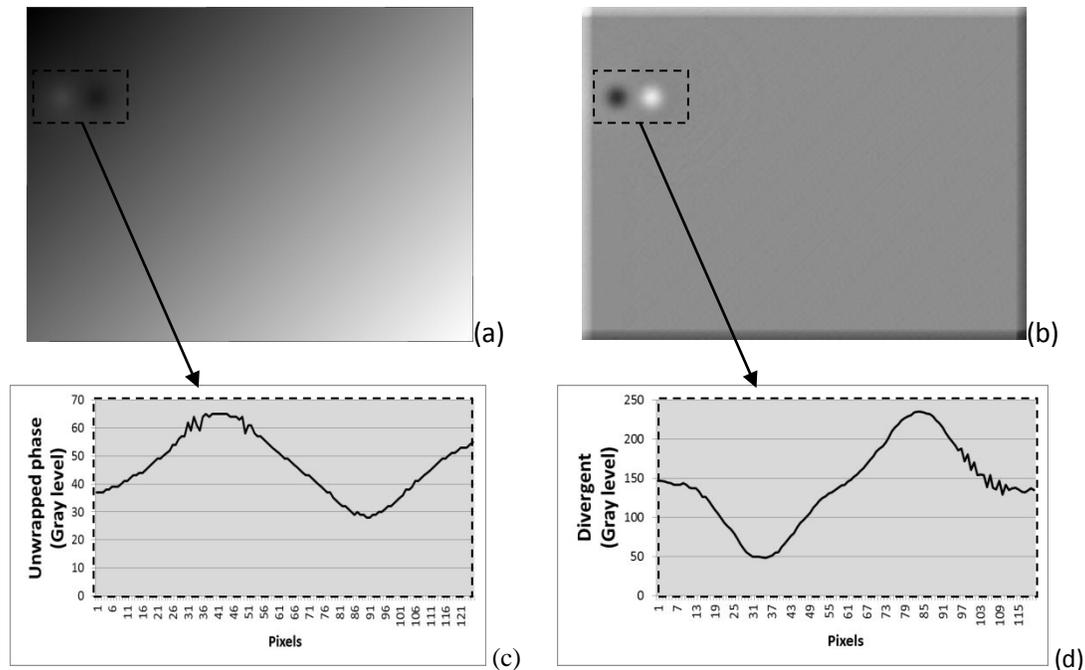
Figure 8: Image processed: (a) Spatial phase unwrapping algorithm, (b) Divergent algorithm, (c) Unwrapped phase profile, (d) Divergent profile
