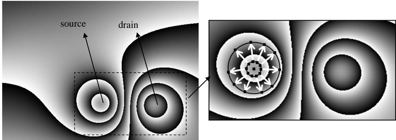
Figure 4: (a) Synthetic phase image with a “butterfly” pattern, (b) A pixel in the image and a set of neighboring pixels symmetrically distributed over a ROI defined by two concentric circles. The arrows show the correspondence between two pixels in the same angular position at the ROI.
