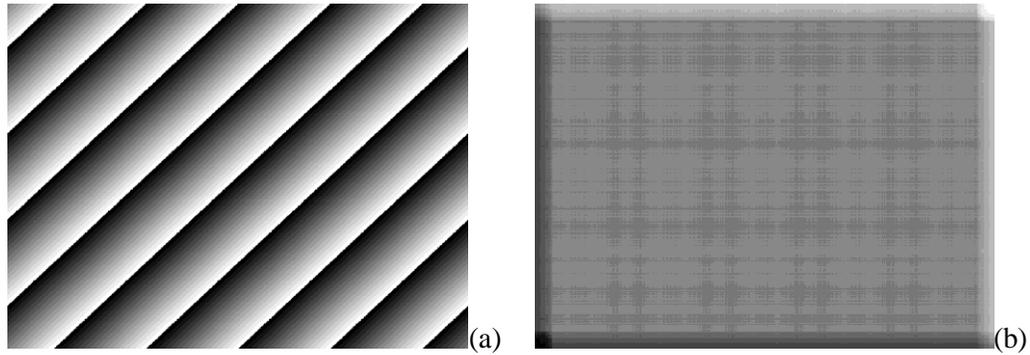
Figure 6: (a) Synthetic phase map of a regular fringe pattern, (b) Processed image
