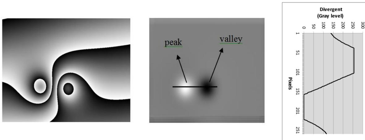
Figure 5: Phase map with an artificial defect, a divergent map and phase profile on the defect region.
