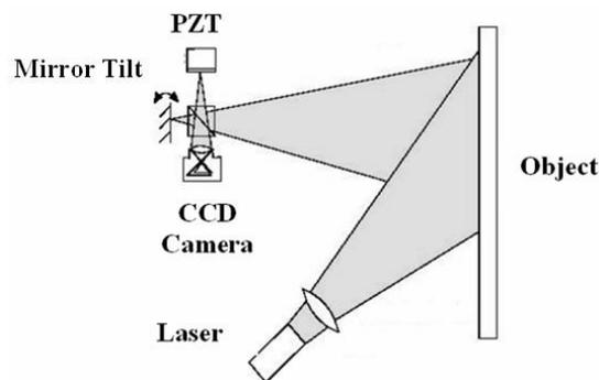
Fig. 2. Shearography set-up.
